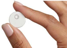
The Libre Duo dual glucose-ketone sensor (Image courtesy of Abbott)
