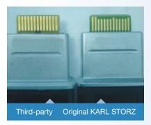
The third-party card edge (left) is noticeably different from the original KARL STORZ component (right). Third-party camera head repairs like this one could have a negative effect on image quality and communication with other devices.
