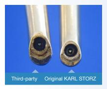
The difference between the third-party shaft and objective assembly (left) and the original KARL STORZ instrument (right) is clear to see. The third-party assembly could degrade the magnification and focus of the image. It may also change the length of the endoscope. Equally important: the seals may not withstand sterilization.
