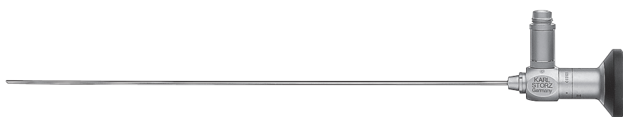
26008BA HOPKINS® Forward-Oblique Telescope 30° , diameter 2 mm, length 26 cm, autoclavable , fiber optic light transmission incorporated, color code: red
